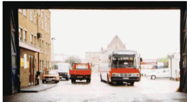
**Figure 8** Bus garage with doors open so as to provide a steady flow of clean air
