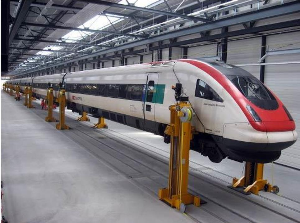
Mobile column lifts are not installed; they are fully mobile, so care must be taken when positioning them. Use a level, hard surface - concrete is best not tarmac. They normally engage with the vehicle's wheels using forks, so take care that the fork is the correct size for the tyre diameter, it's also worth checking that the tyre pressure is correct.
